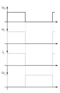
Elementary transistor circuits - freewheeling diode
